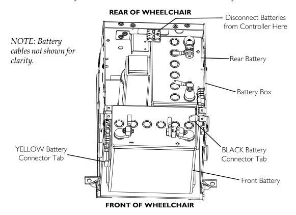
FIGURE 10.3 Removing the Batteries
